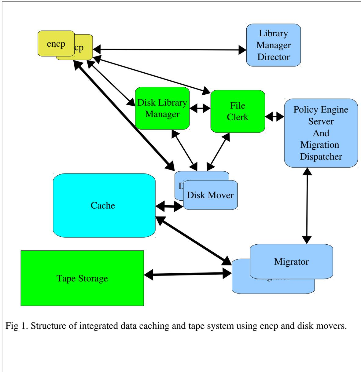
Fig 1. Structure of integrated data caching and tape system using encp and disk movers.
