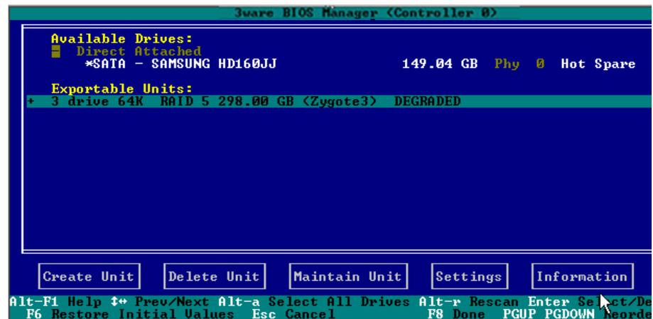
You can start the rebuild of a degraded unit manually in 3BM, or you can let the system boot and allow the rebuild to take place automatically.
