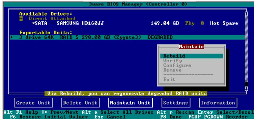
The Rebuild Disk Array screen displays.
